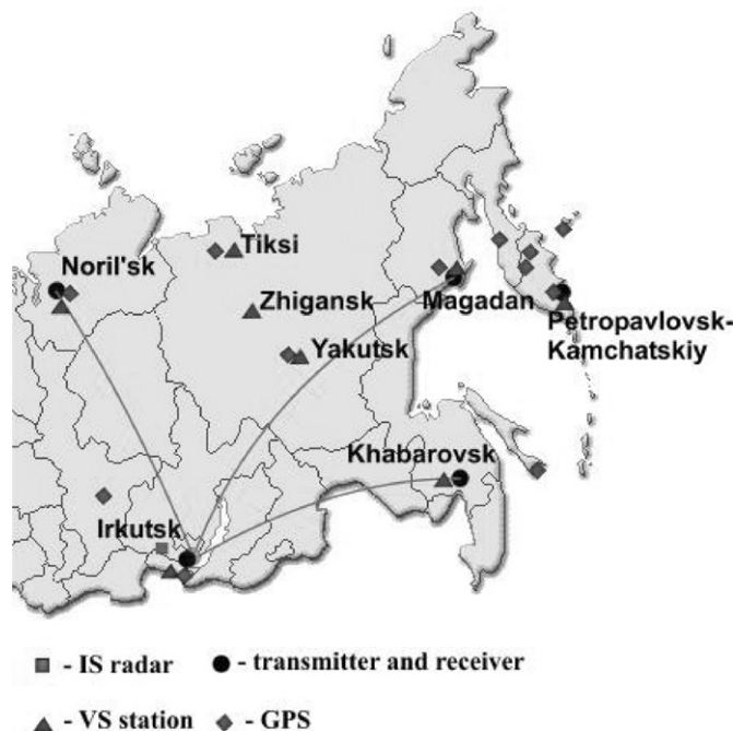
Fig. 1. The location of ionosondes, the oblique-incidence sounding paths and the types of experimental equipment.
