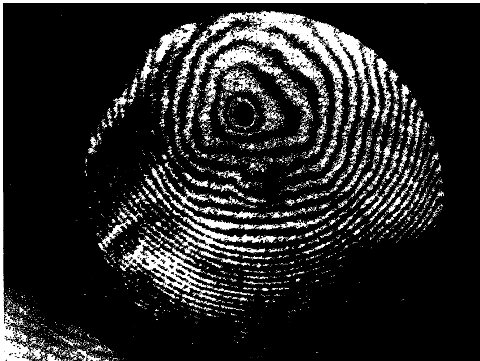
Fig. 7. Interference between the two surfaces of the entrance window.
