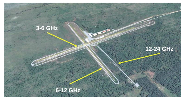
Figure 1. Schematic arrangement of antenna arrays of the Siberian Radioheliograph
